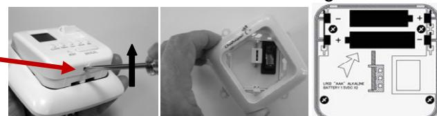
Hinge the timer unit upwards and carefully detach, (note – there is also a lug at the top). Then lift the timer surround and rotate slightly so that it can be removed (see picture). At this stage **insert the two AAA cells** in the timer module. The polarity is shown underneath the batteries – it is easiest to insert the outermost battery first, then the inner one – note that the two batteries are installed in opposite directions!
