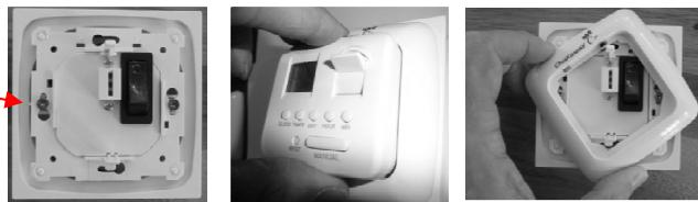
Then position the frame over the front (Chuxaway label uppermost) rotating it slightly to clear the upper and lower retaining lugs. When the surround is flush against the faceplate, carefully push the timer module into place, hinging slightly backwards as you push it into place (so that the top lug clicks into place just before the bottom). If you struggle with this step then it may help to slightly loosen the two threaded screws, as the base can warp if these are over tightened.
