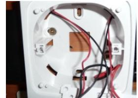
Thread the wires from the motor and battery packs through into the control unit housing. Either feed the cables though holes in the rear of the control unit housing, or from the side as shown in the picture. Fix the control unit housing in place using two of the large screws (supplied).
